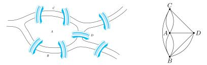
The problem asks for building an Euler circuit. It it not possible because the graph representing the problem has vertices of odd degree (e.g.  $\delta(A)=5$ ).
